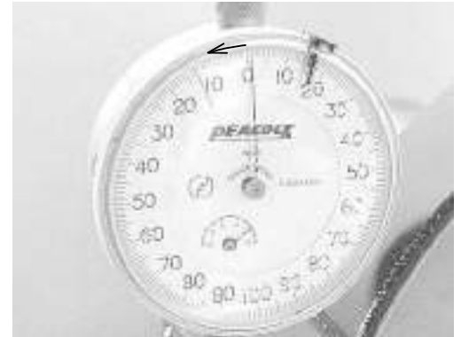
Fig. 1.11 Setting the GN Gauge
